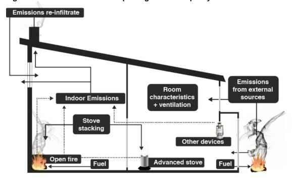
Figure 1. Schematic of factors impacting indoor air quality
