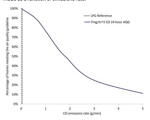
Figure 8. Percentage of modeled kitchens with chimney stoves predicted to meet CO AQGs as a function of emissions rate.
