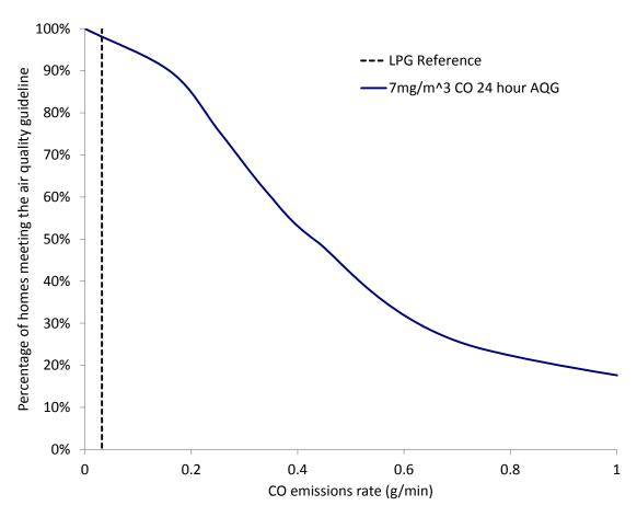
Figure 6. Percentage of modeled kitchens predicted to meet CO AQGs as a function of emissions rate.
